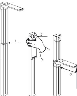
2. Push measuring slide upwards according to the height of the person to be measured.
