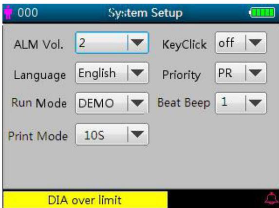
Figure 4.22A System Setup Screen
