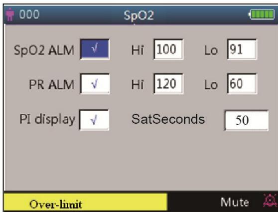
Figure 4.12C SpO<sub>2</sub> Setup Screen (with Nellcor SpO<sub>2</sub> configuration)
